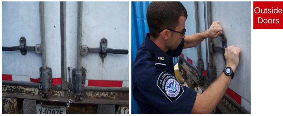
Check Locking Mechanism Bolts / Rivets Secure
